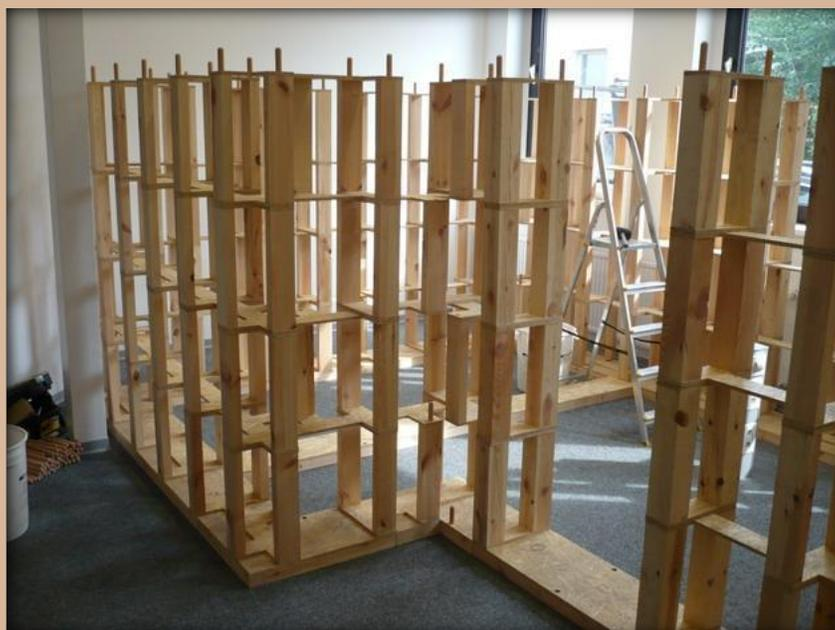
Img. 3 Walls without insulation – tests in HSW Institute (Germany)
